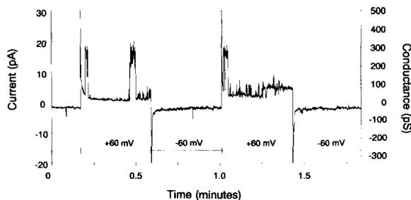
Figure 4. Individual, Large (220 pS) Channels Are Gated Open in Low (0.2 nM) Concentrations of Signal Peptide
